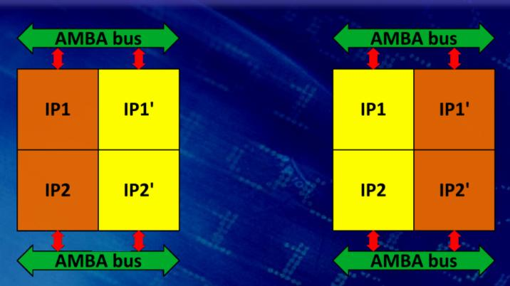
By ensuring the 50% probability of having '0' in each configuration memory bits, by switching among two status (Work and Rest), providing the minimum aging effect [5] increasing the SNM
