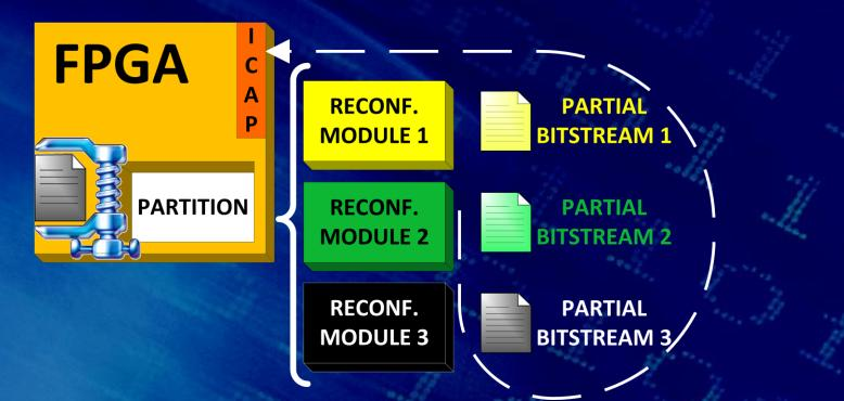
A special partial bitstream, for each reconfigurable partition, is compressed and stored internally the FPGA, to quickly reconfigure if a faulty bitstream has been read
